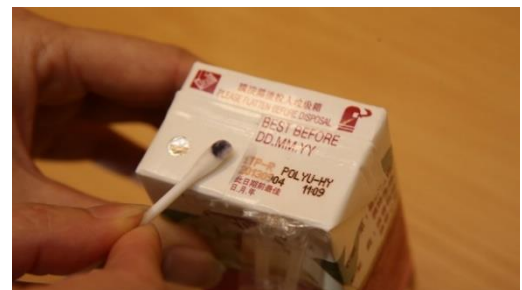
Fig. 1) Drink carton with nano-ink: tampering has revealed orange double layer
