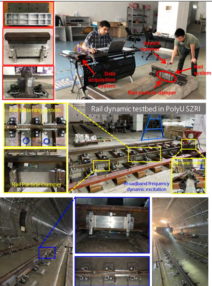
Figure 2: Laboratory and field experiment investigations and verifications
