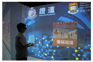
Dr Henry Y.K. Lau of the Department of Industrial and Manufacturing **Systems** Engineering and his team have developed the technology, imseCAVE creating interactive virtual reality environment with multi-screen stereographic projection and multiple object tracking capability that is powered by a customizable and configurable virtual reality engine. It is an innovative solution that creates lifelike objects and scenarios without the limits of time and space
