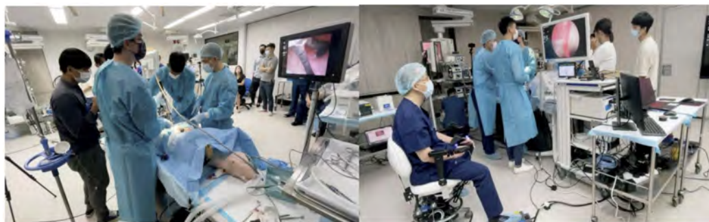
Fig. 30. The flexible miniature surgical robot in animal study including patient-side setup and surgeon's master console.
