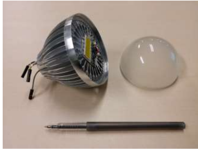
Fig. 6.1.2.4. Prototype of the high performance LED lighting system by wafer level integration.
