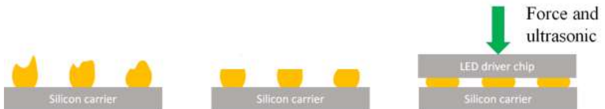
Fig. 6.1.2.2. Au stud flip-chip bonding process: Au stud bumping (left); coining (middle); bonding (right).
