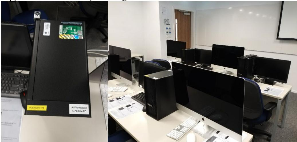
Purchased a deep learning central machine in March 2021. This central machine is being upgraded to accommodate 8 high-performance GPU's and a large amount of fast memory to run deep learning with big data available locally in the machine. This central machine is used for intensive deep learning tasks which can take over one week for each task even with a dual GPU machine.
