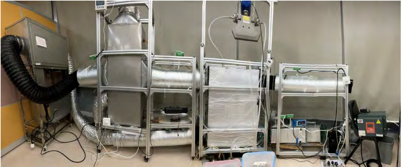
Figure 1 Test Rig for Desiccant-enhanced Evaporative Cooling System Experiments
