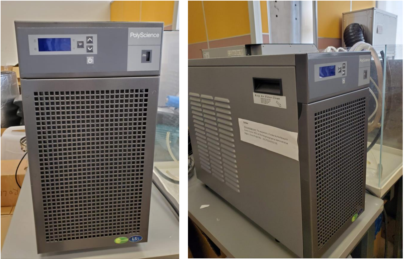
Figure 6: Cooling Water System (Chiller)
