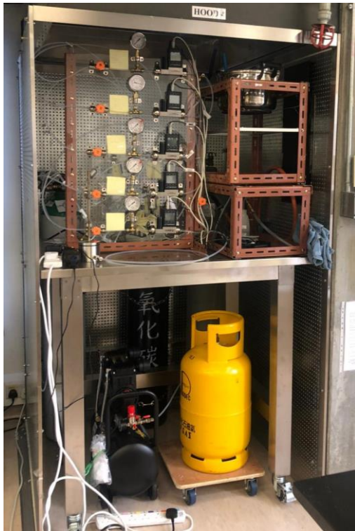
Figure 1: Test Rig for Premixed H 2 /LPG/Air Combustion Experiments
