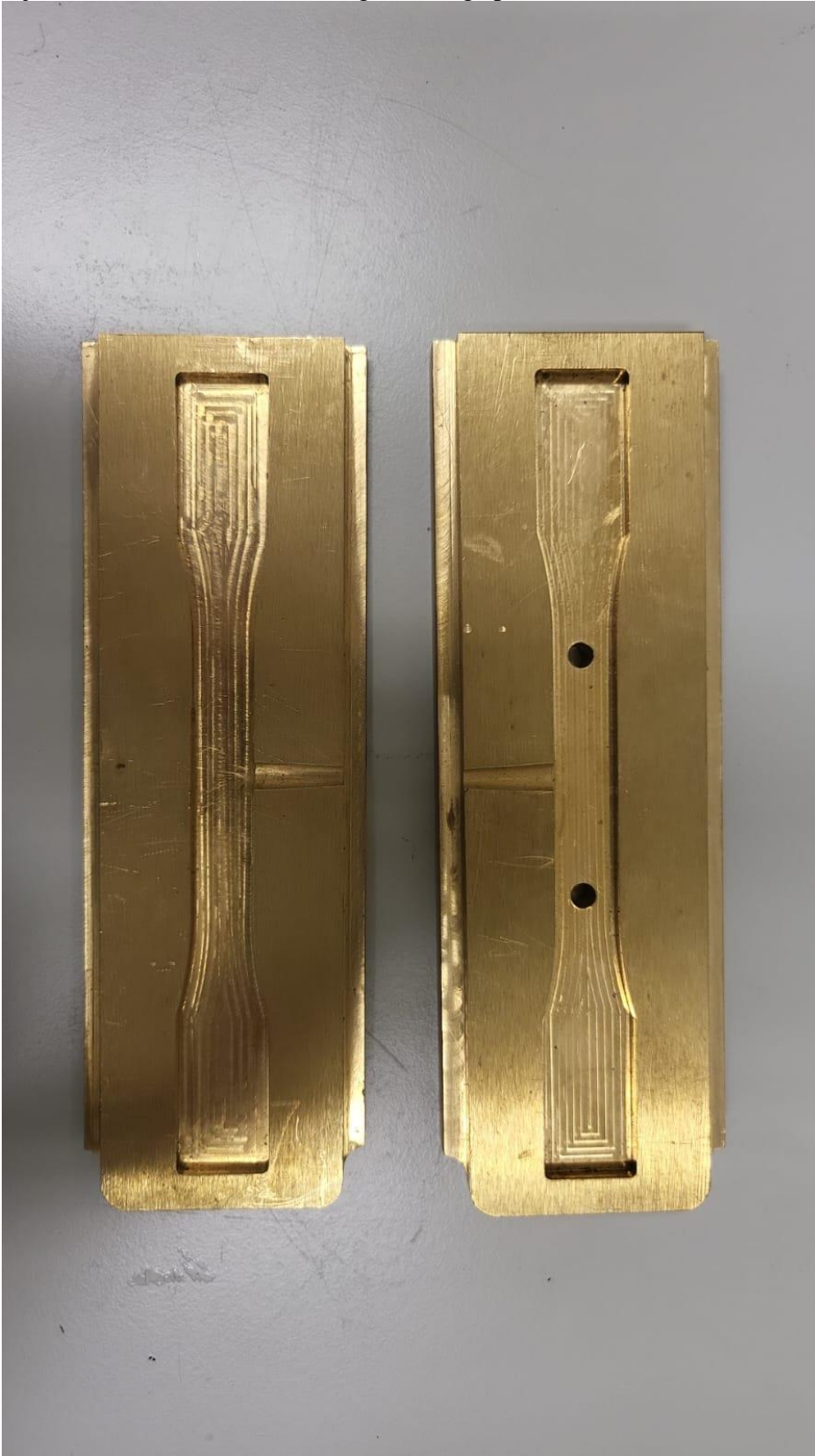
Injection mould - Tension strength testing specimen.
