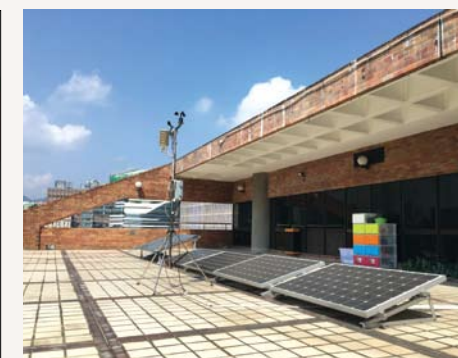
An isolated microgrid laboratory is established with stand-alone or grid-connected mode, powered by either PV or the utility grid, overall power capacity reaches 4 kW. 團隊設立之智能微電網實驗室總容量達4 kW，能獨立或與多個電網並網操作；能自行以光伏供電，亦能與電力公司電網並網運行。
