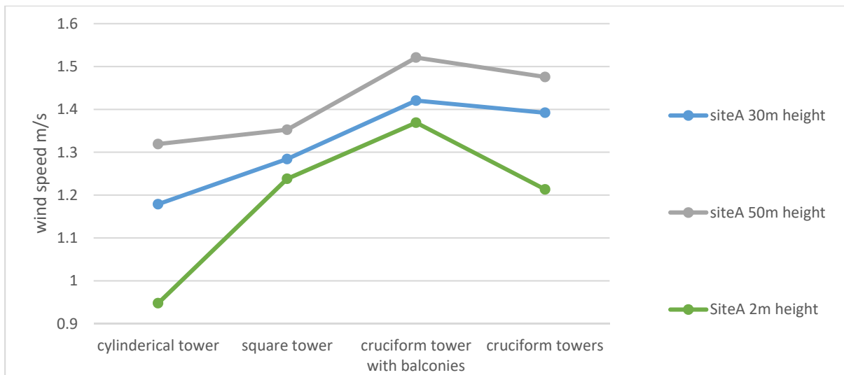
Figure 6: Building geometry impact on wind speed at different height zones (Authors et al. 2016)
